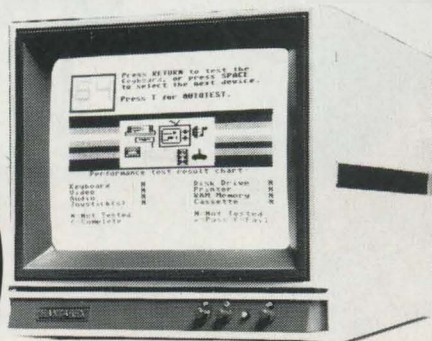
CT2000 12'' High Resolution Monochrome Monitor L1 - orange skjerm 18 Mhz båndvidde
